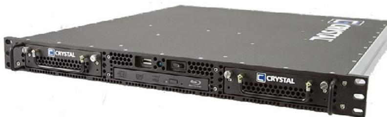
*The RS112 1U rugged server meets MIL STD 810 for shock, vibration, and temperature limits.*
