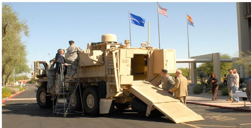
*Prophet provides the tactical commander with an enhanced capability for electronic intelligence preparation of the battlefield, battlespace visualization, target development and force protection. Crystal Group's RS112 1U rugged server located inside Prophet vehicles provides data analysis and other tasks in a battlefield environment.*
